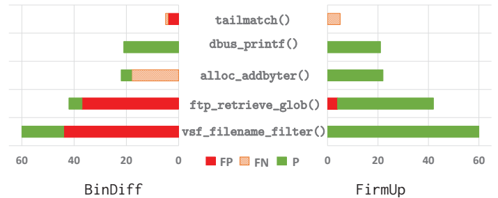
Figure 6. Labeled experiment comparing BinDiff with FirmUp, showing that BinDiff encountered over 69.3% false results overall compared with 6% for FirmUp
